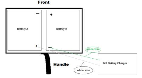
Attach the *white wire* on the MK Battery Charger to the positive terminal on Battery A. Attach the *green wire* on the MK Battery Charger to the negative terminal on Battery B.
