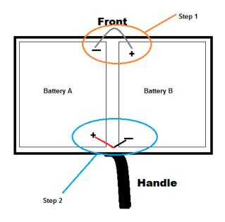
**Step 1:** Connect the negative terminal of Battery A to the positive terminal of Battery B using an inline fuse (or wire). This will hook the batteries in series.
