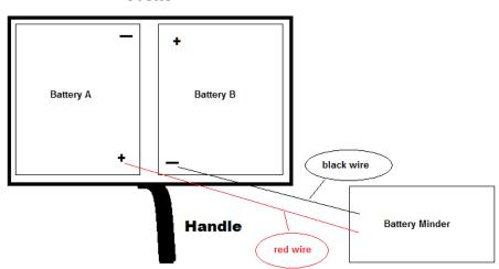
Attach the *red wire* on the BatteryMinder Charger to the positive terminal on Battery A. Attach the *black wire* on the BatteryMinder Charger to the negative terminal on Battery B.
